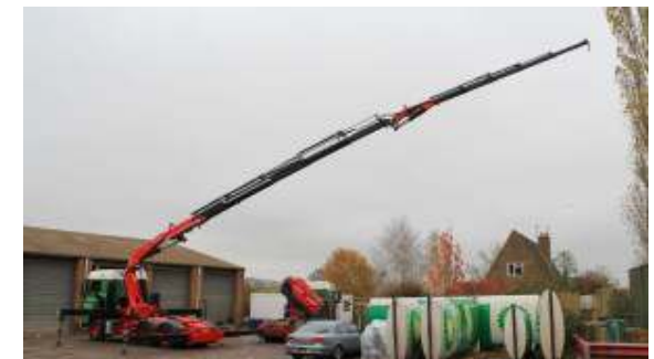
80 tonne/metre crane with fly jib 24m reach
